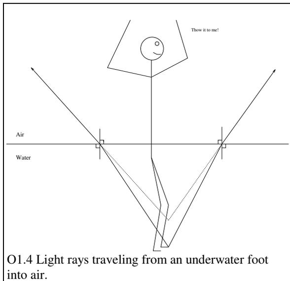
We must not work from the eye to the object. We must start with the source of the light. We can see that once the light is traveling
