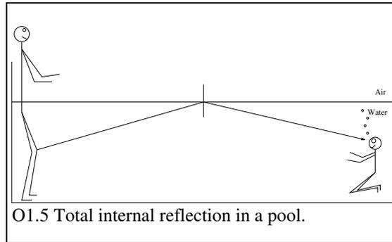
If the incident angle is larger than the critical angle, where does the light ray go? The light ray does not enter the second medium but reflects off the boundary between the two media as if there was a mirror located at the interface. The fundamental *why* of this phenomena is beyond our ability at this point but this is
