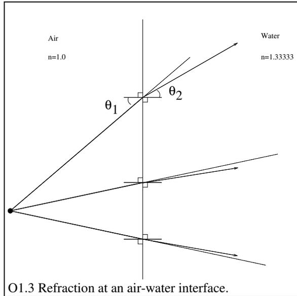
This bending of light is very common and very easily observed with fish tanks, water glasses, swimming pools, and streams. Refraction is responsible for the making straws look bent in water glasses and it is responsible for making your legs look shorter when standing in the water.
