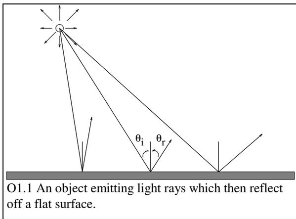
situation that is in effect for the typical bathroom mirror. In real situations there are absolutely oodles and oodles of light rays hitting the mirror with a vastly huge variety of angles and positions. Yet every ray behaves according to  $\theta_i = \theta_r$ , so in order to understand the mirror we only need to look at a few rays.
